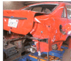
Full body sectioning is more commonly used when the damages to the rear of the vehicle would require extensive rear floor replacement/repair along with the rear frame rails, one or both rear quarter panels, the rear body panel and the rear outer cosmetic panels. These types of damages often start the "total loss" calculators buzzing while makin unqualified "rebuilders" salivate.
